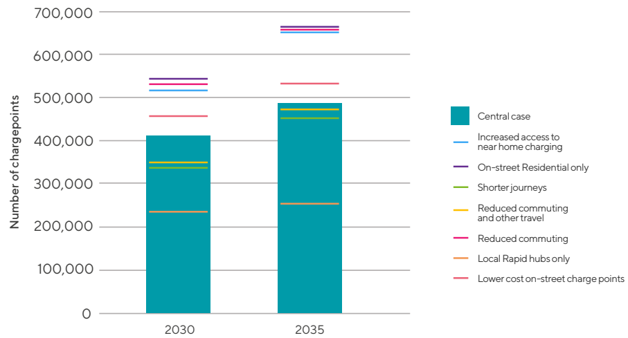
Figure 10 – Total number of UK public chargepoints (2030 and 2035) and impact of variations to: availability of near home charging; journey lengths; overall vehicle mileage; and upfront costs of on-street residential chargepoints.
